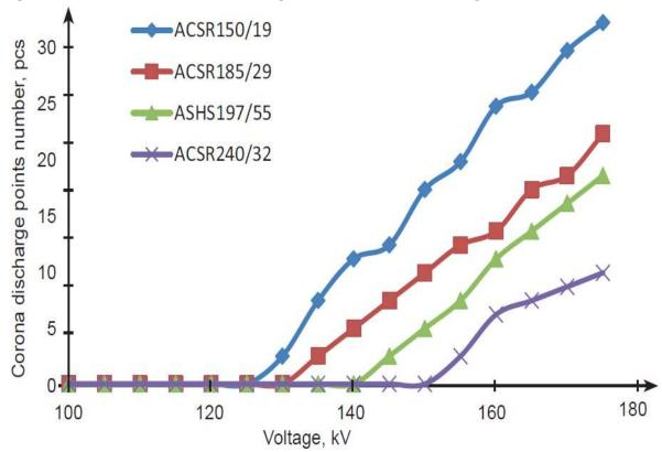
Fig. 5. Dependence of corona discharge points number on voltage
