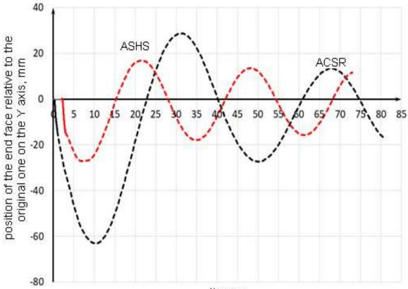
**Fig. 3.** Change in time of a vertical coordinate of a free end face of a piece of ASHS 128/36 and ACSR 120/27 wires at damping fluctuations.
